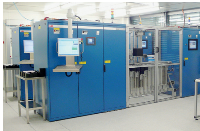
Automated IGBT and diode dies test system
