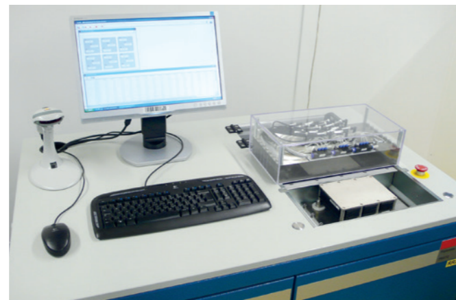
Baseplate flatness tester. Mechanical measurement under pressure (resolution up to 0.1 micrometer)
